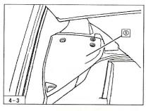
4. Install the upper cover of the rear damper ①.(Diagram4-3) \*Do not reuse the removed rear damper cap ② in the diagram 3-2. Secure the upper cover of the rear damper ① using a clip and a screw. The factory cover is secured using a clip and 3 screws.
