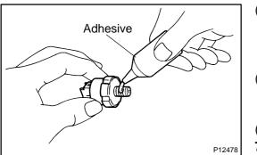
(c) Apply adhesive to 2 or 3 threads of the oil pressure switch. Adhesive:
