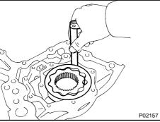
Standard body clearance: 0.100 - 0.175 mm (0.0039 - 0.0069 in.) Maximum body clearance: 0.20 mm (0.0079 in.) If the body clearance is greater than maximum, replace the ro-
