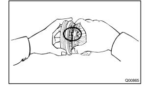
(c) Using a press, install the 3rd gear and No. 2 clutch hub.
