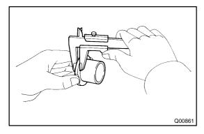
(b) Using vernier calipers, measure the inner race flange thickness.
