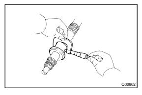
(c) Using a micrometer, measure the outer diameter of the output shaft journal.
