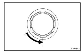
(c) Install the synchronizer cone ring to the reverse synchronizer pull ring and turn the pull ring.
