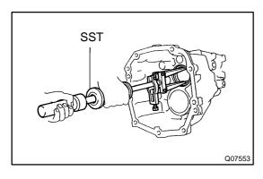
(b) Using SST, remove the outer race. SST 09308-00010
