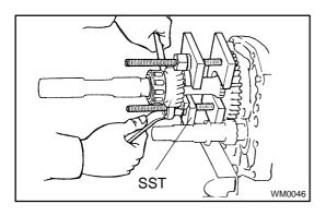
(b) Using SST, remove the rear bearing and 5th gear. SST 09312-20012 (09313-00030, 09313-00040, 09313-00050)
