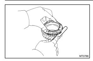
(d) Using a feeler gauge, measure the clearance between the synchronizer ring back and the gear spline end.
