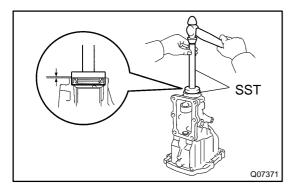
(b) Using SST and a hammer, drive in a new oil seal. SST 09950-60010 (09951-00560), 09950-70010 (09951-07150)
