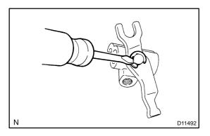
(o) Using a screwdriver, remove the E-ring, separate the reverse shift head and reverse shift arm.
