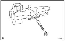
(c) Using a hexagon wrench (10 mm), remove the straight screw plug.
