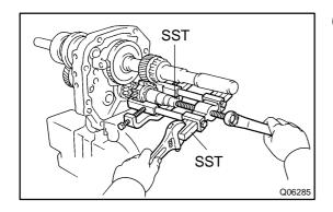
(d) Using SST, remove the No. 3 clutch hub. SST 09950-40011 (09951-04020, 09952-04010, 09953-04020, 09954-04010, 09955-04051, 09957-04010, 09958-04011) 09950-60010 (09951-00200)
