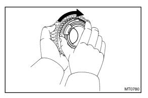
(c) Check the braking effect of the synchronizer ring. Turn the synchronizer ring in one direction while pushing it to the gear cone. Check that the ring locks.
