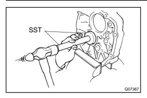
(c) Using SST and a hammer, tap out the bearing outer race. SST 09950-60010 (09951-00510), 09950-70010 (09951-07150)
