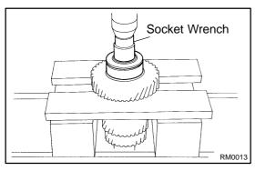
(e) Using a socket wrench and press, install a new bearing, side race and inner race.
