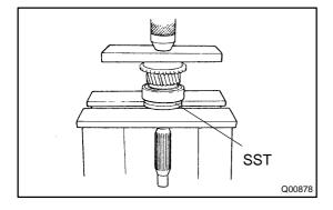
(c) Using SST and a press, install a new bearing. SST 09506-35010
