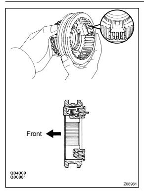
(g) While pushing 3 shifting keys, install the synchronizer ring assembly to the No. 3 hub sleeve.
