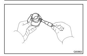
(d) Using a micrometer, measure the outer diameter of the inner race.
