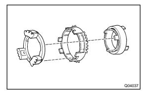
(c) Remove the reverse synchronizer ring and 5th synchronizer ring from the synchronizer pull ring and cone ring.
