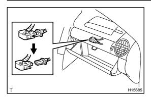
(b) Disconnect the front passenger airbag assembly connector.
