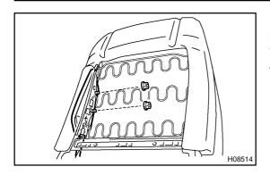
(3) Remove the 2 nuts and side airbag assembly. **CAUTION:**
