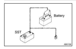
(c) Check functioning of the SST (See step 1-(a) on page RS-14).
