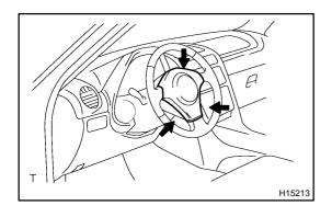
There should be no interference between the steering wheel pad and steering wheel, and the clearance should be uniform all the way around when a new steering wheel pad is installed on the steering wheel.
