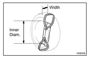
(3) Position the side airbag assembly inside the tire with the airbag deployment direction facing inside. Tie the side airbag assembly to the tire, as shown in the illustration.
