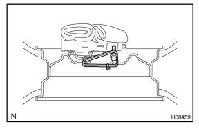
(3) Face the upper surface of the steering wheel pad upward. Separately tie the left and right sides of the steering wheel pad to the disc wheel through the hub nut holes. Position the steering wheel pad connector so that it hangs downward through a hub hole in the disc wheel.
