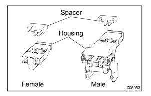
(1) Terminal twin-lock mechanism: Each connector has a two-piece component consisting of a housing and a spacer. This design enables the terminal to be locked securely by two locking devices (the retainer and the lance) to prevent
