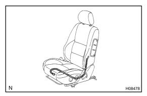
(b) Disconnect the side airbag assembly connector.
