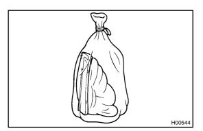
(g) Dispose of the side airbag assembly.
