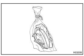
(i) Dispose of the steering wheel pad (with airbag).
