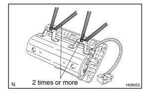
(1) Pass the wire harness through the installation holes, as shown in the illustration.
