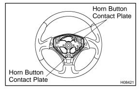
Check the deformation of the horn button contact
