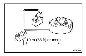
(2) Move the SST to at least 10 m (33 ft) away from the steering wheel pad tied down on the disc wheel.
