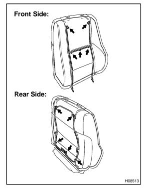
(2) Remove the 10 hog rings, headrest supports and seat back cover, as shown in the illustration.
