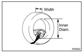
(2) Position the front passenger airbag assembly inside the tire with the airbag deployment side facing inside. Tie the front passenger airbag assembly to the tire, as shown in the illustration.
